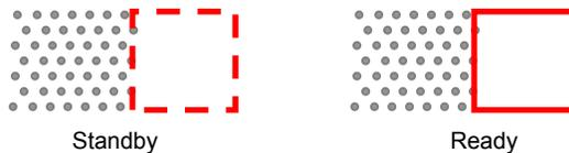
Care should be taken to apply adjoining scans without gap or excessive overlap of the previously scanned area. Line each scan pattern up to each other to avoid gap or overlap as shown above.
